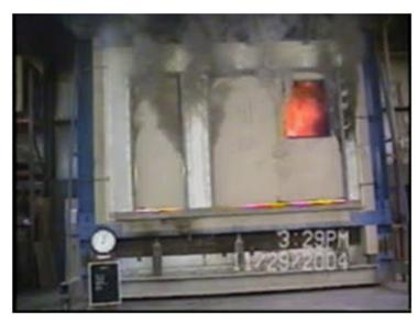
20-minute fire-rated Acrovyn Door being tested by ITS/WH.
