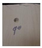
High Pressure Laminate 4 in lb failure
