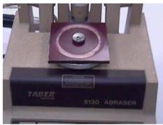
Wood Veneer w/ Stain and varnish failed sample - 1,000 cycles.
